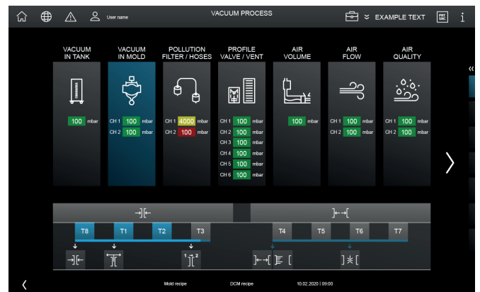
Figure 6: Overview of the Fondarex Modular control panel showing the main control points of the vacuum process
